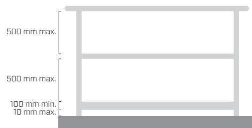
without curb or less than 150 mm
