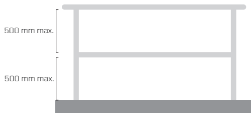
with curb greater than 150 mm
